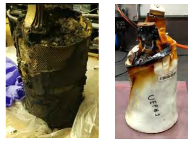
UEP Zn-MnO 2 batteries after 9540A testing (above) and temperature data captured during the test (below)
